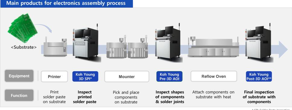
\* SPI: Solder Paste Inspection \*\* AOI: Automated Optical Inspection
