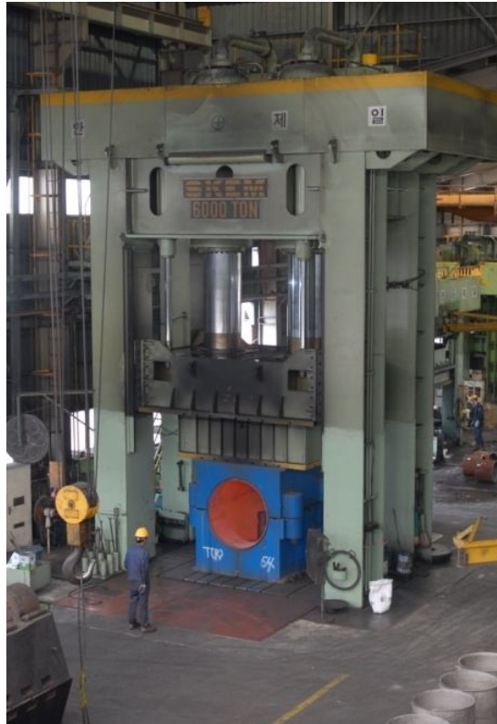
5,000 Ton Hydraulic Press
