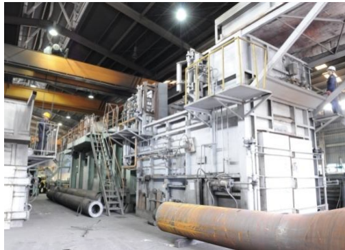
Hot Forming Elbow Machine
