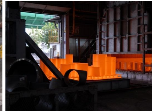
Solution Heat Treatment Furnace
