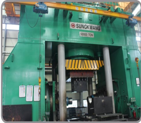
50,000TON TEE BULGING PRESS
