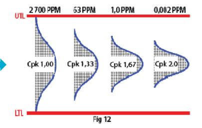
What is Cpk: Statitical measure of process capability; the ability of a process to produce Output within specification limits.
