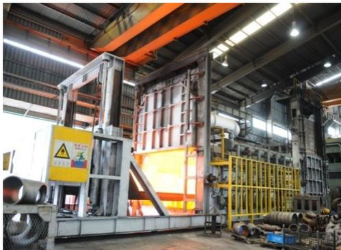
Heat Treatment Furnace For Fitting
