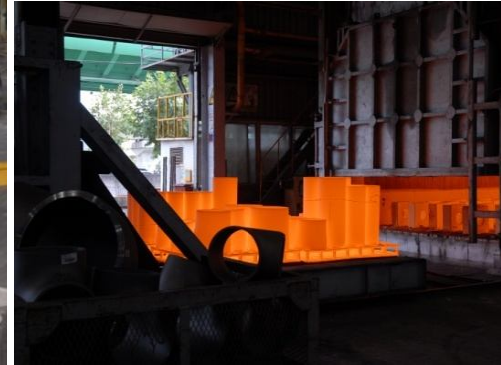
Solution Heat Treatment Furnace
